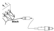
4. Connect the Audio Adapter's red power wire (with inline fuse holder) to a point in your vehicle's fuse block that has power only when you turn the vehicle's key to either the accessory (ACC) or START position.
